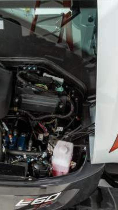
Bobcat makes it easy to find and reach your engine checkpoints in a Bobcat excavator so daily maintenance actually gets done every day. Comparing our service access to other excavators is like comparing a 60-inch LCD to a 15-inch black-and-white TV. The swing-open tailgate and side access hood put the engine and pump package, valve bank, cooling system, and plumbing in easy reach.
