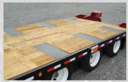
"LP" (Low-Profle) models feature a 10-inch beam, steel over the wheels, and a 12° beavertail for a lower deck height.
