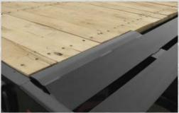
Wood protectors are standard on Towmaster T-series trailers. They protect the end of the deck boards when loading equipment.
