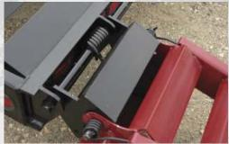
Two-way spring-assist ramps allow easy lifting of ramps off the deck and the ground. Grommet mounted LED lights are standard.
