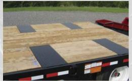
"LP" (Low-Profle) models feature a 10-inch beam, steel over the wheels, and a 12° beavertail for a lower deck height.
