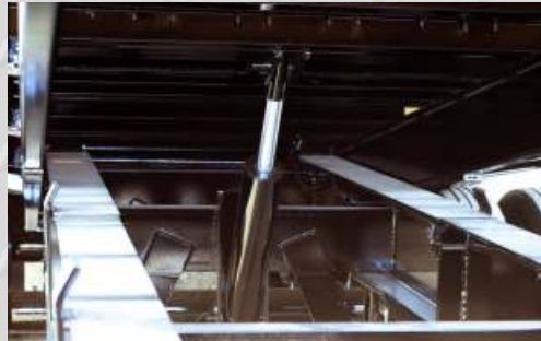
Cushion cylinder controls the deck tilt when loading or unloading equipment. Optional Hutchens® 9700 suspension shown.
