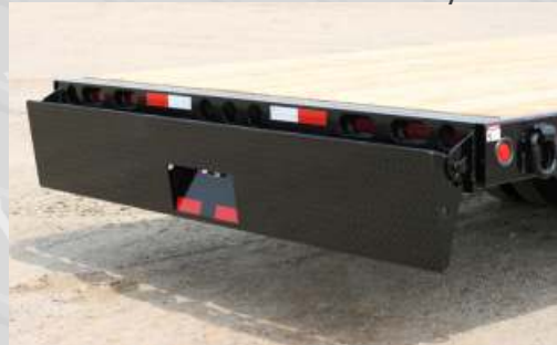
Patented automatic kick-out ramp doubles as under-ride protection.
