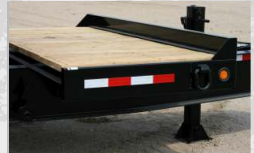
4-foot stationary deck is standard and allows room for longer equipment and the added length makes towing easier.
