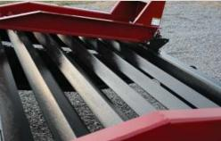
Self-cleaning angle iron beavertail provides positive traction when loading equipment.
