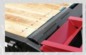
Wood protectors are standard on Towmaster T-series trailers. They protect the end of the deck boards as equipment is loaded.
