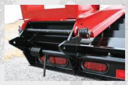
Two-way spring-assist ramps allow easy lifting of ramps off the deck and the ground. Grommet mounted LED lights are standard.
