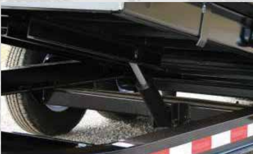
Cushion cylinder controls the deck when loading or unloading equipment.
