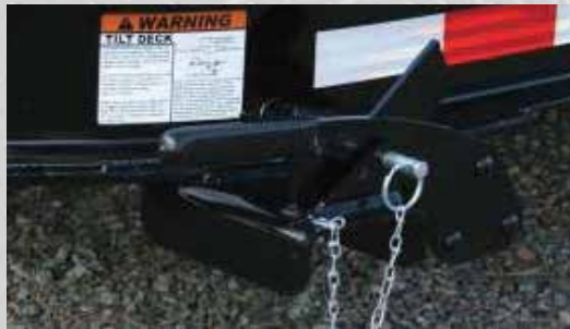
Single deck lever with dual latch securement is easy to operate.
